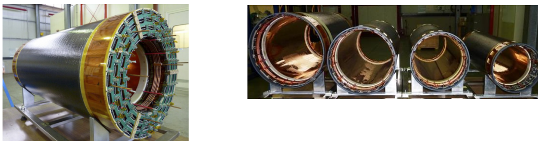
Figure 1. The Inner Tracker detector before its installation in the KLOE-2 interaction region is shown in the left panel. All the four layers before assembling them to build the Inner Tracker are shown in the right panel.
