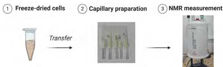
FIGURE 5.8: Scheme presenting workflow of NMR measurement. Freeze-dried WM266-4 cells in the capillary for NMR studies. The number on capillary denotes given freezing medium as in 5.4.1. Created with BioRender.com
