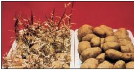
Fig 8. Illustration of how the sprouting losses in stored potatoes can be prevented by irradiation with a dose of 200 Gy. In Japan potatoes have been irradiated industrially already since 1973. The figure is taken from [17].
