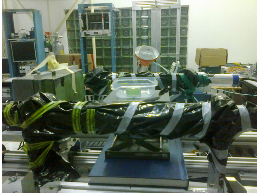
Figure 6.1: Picture of a phantom used for measurement, inside one can see pan with the source.
