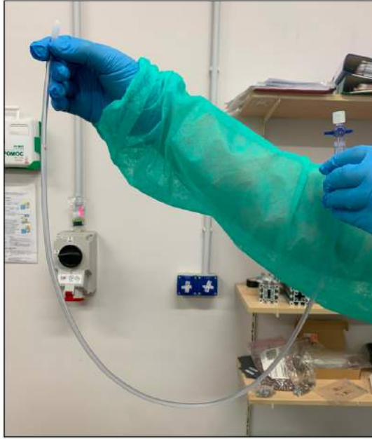
Figure 7.4: (Right ): Display the 70 cm tube that uniformly filled with a water solution containing ^{18}\text{F} isotope with a well defined activity. (Left): Schematic decay of the ^{18}\text{F} . Figure adapted from [112].
