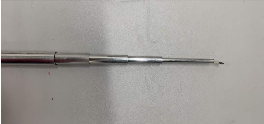
Figure 4.1: Sensitivity Phantom with five sleeve tubes and one polyethylene tube (sixth layer) with length of 70 cm.
