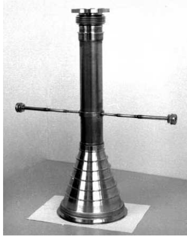
Figure 3.5: Beryllium scattering chamber together with a thin pipe for the pellets stream.
