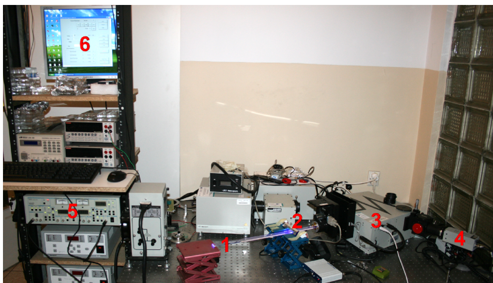
FIGURE A.2: The measurement setup: 1) the scintillator, 2) the UV lamp, 3) the monochromator, 4) the detector, 5) the lock-in amplifier, 6) the computer to control the monochromator
