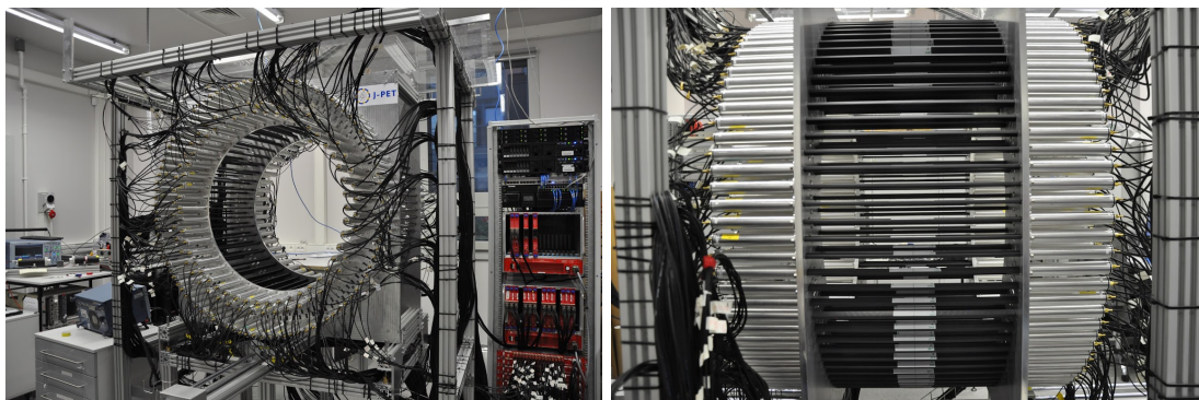
FIGURE 2.4: The three-layer 192-strip J-PET prototype, colloquially called the "big barrel". (left) Photography of the laboratory with the J-PET prototype. The detector is visible in the main plan. Also the rack with the computing units and the high voltage power supplies is visible in the right part of the photography. (right) Scintillator strips are covered with the black Pokalon foil and mounted between two square aluminum plates. Aluminum tubes outside the detector chamber are the slots for the photomultipliers.
