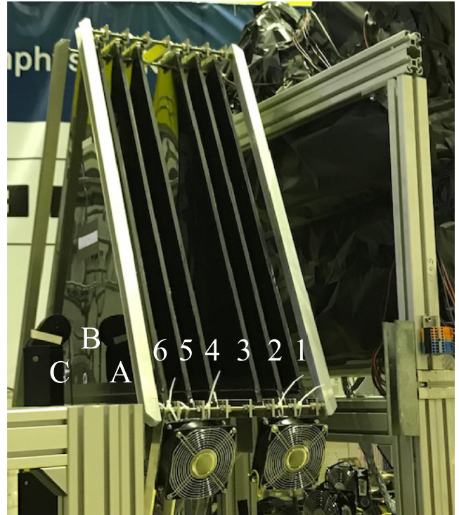
Fig. 6. Arrangement of the iTOF-modules for measurements with proton beam and cosmic particles. For the tests with cosmic particles the stack was rotated by 90^\circ .
