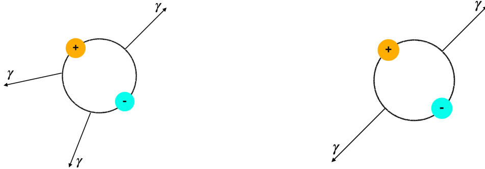
Figure 2.4: Schematic depiction of positronium decay into ( left ) three and ( right ) two gamma quanta.
