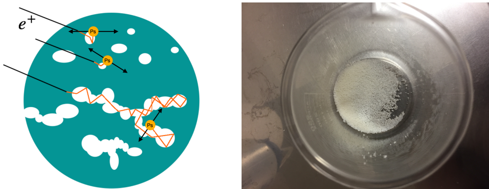
Figure 2.7: Left: Schematic representation of different sized pores in XAD4 and ortho-positronium paths. Right: Sample of dried XAD4 used in the measurements in a beaker.
