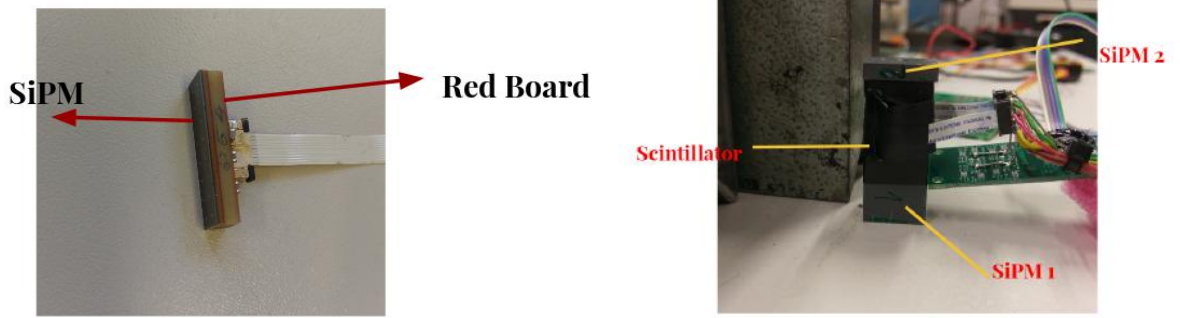
Figure 4.18: (left) Pictorial representation of SiPM mounted on red board. (right) Representation of test setup consisting of a light-tight container with scintillator and SiPMs inside.
