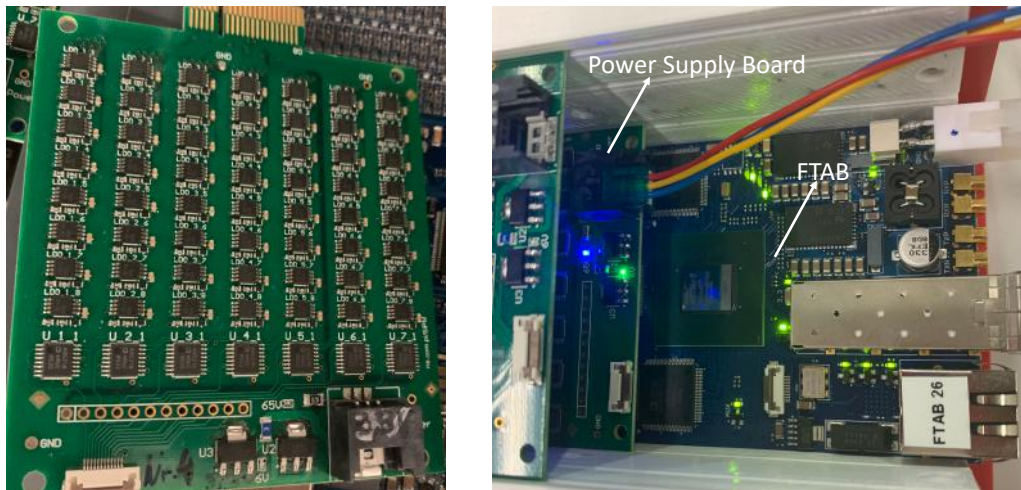
Figure 4.24: Power supply board (left) and Power supply board and FTAB inside the detector.
