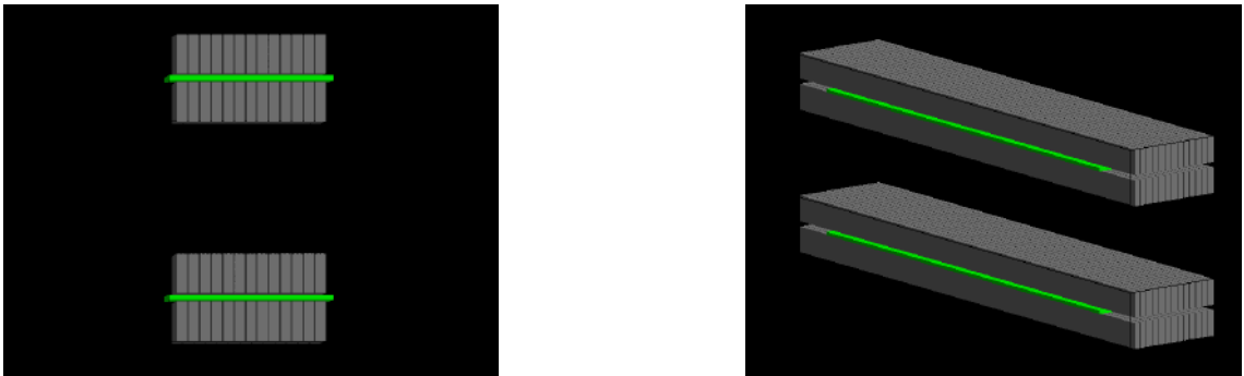
Figure 5.1: The figures illustrate the geometric configuration of the JPEM detector in different orientations. In the diagrams, the WLS (Wavelength Shifting) material is represented in green colour, while the plastic scintillator is depicted in grey. The left figure specifically presents the detector geometry in the x-y cross-section.
