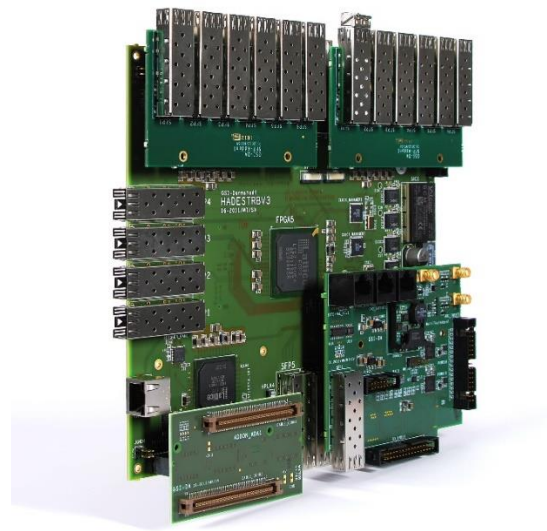
Figure 23: Photo of TRB3 equipped with different extension modules. On top there are two SFP mezzanine Add-ons plugged, down left is an ADA mezzanine Add-on and on the down right Multi-test mezzanine Add-on. [trb.gsi.de]
