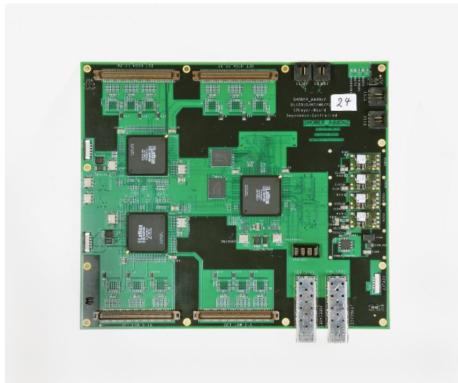
Figure 38: Photo of Shower Add-on board. Four brown connectors deliver analog signals to ADCs which are controlled and read out by the FPGAs. One central FPGA is a controller and an interface to both TrbNet and Gigabit Ethernet network, through the optical connectors.
