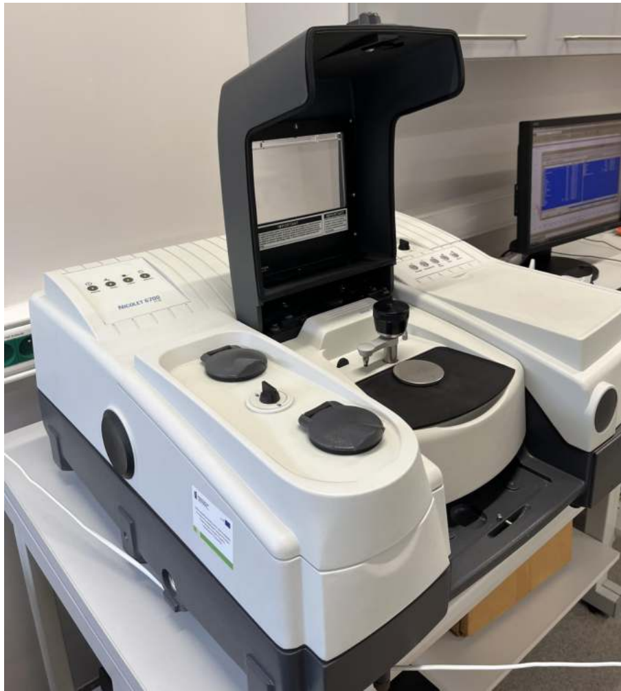
Figure 10. Nicolet 6700 (ThermoFisher Scientific, MA, USA) FTIR-ATR spectrometer, Department of Medical Physics, Institute of Physics Jagiellonian University, Kraków, Poland.
