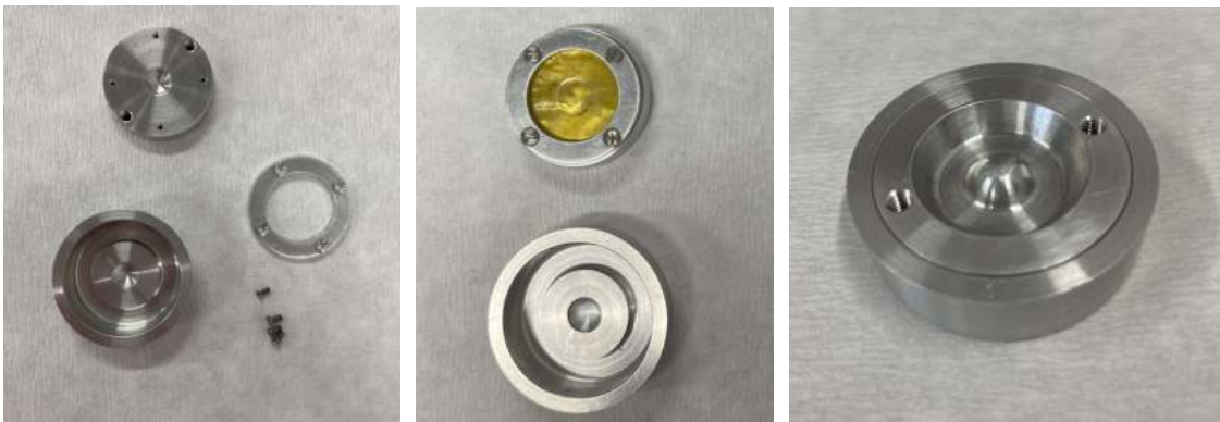
Figure 14. Measuring chamber; it was specially designed so that it is possible to perform measurements even with a small amount of sample. It is spherical in shape with a radius of 7mm and has a total volume of 200 \mu\text{m} (100 \mu\text{m} at the bottom and 100 \mu\text{m} at the top part).
