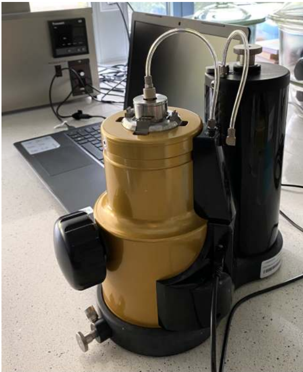
Figure 9. IZON qNano device used to determine the concentration of the EV sample(left); An exemplary nanopore placed on a polyurethane membrane (right) [34].
