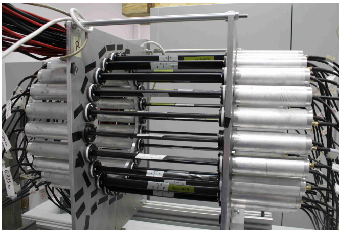
Fig. 3. 24-modules prototype of J-PET scanner. BC-420 scintillators (covered with black foil) were forming single ring with 360 mm diameter. To each side of the scintillator a R4998 Hamamatsu photomultipliers were connected.
