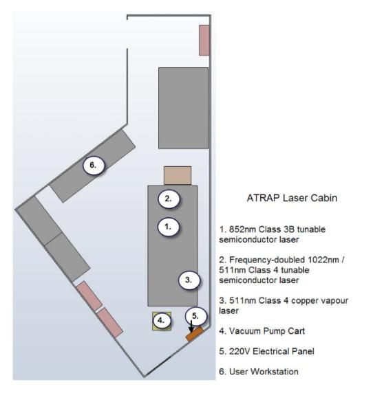
Figure 13: A third Faraday cage contains two laser tables. Our initial laser configuration shown has just been updated to accomodate the pulsed Lyman alpha source described and pictured in the text.
