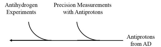
Figure 6: The ATRAP beamline has two antiproton ports – one for antihydrogen experiments and the second for antiproton experiments.
