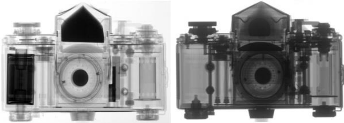
Figure 2. Example of a neutron imaging (left) of an analog camera in comparison with X-ray imaging (right), where neutrons make it possible to see not only heavier materials such as metals, but also some light materials such as hydrogenous substances, plastics etc. (Figure adapted from PSI website (see the link in the references)).
